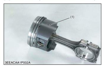
Piston's skirt is coated with **molybdenum disulfied★**, which reduces the piston slap noise and thus the entire operating noise.
