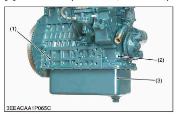
The oil pan is extended under the gear case. Therefore, the height of the engine can be lowered more than so far while securing a necessary amount of oil.
