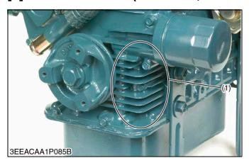
The cooling fin is set up around the oil passage in the gear case.
