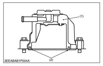
The rubber packing is fitted in to maintain the cylinder head cover 0.5 mm (0.02 in.) or so off the cylinder head. This arrangement helps reduce noise coming from the cylinder head.
