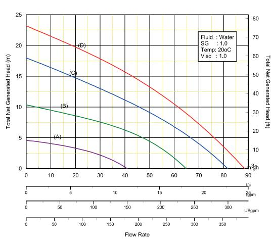
Hydraulic Input: (A) 11 I/m @ 48 bar (B) 19 I/m @ 107 bar (C) \* 26 I/m @ 145 bar (D) 30 I/m @ 172 bar \* Typical performance with HT25D
