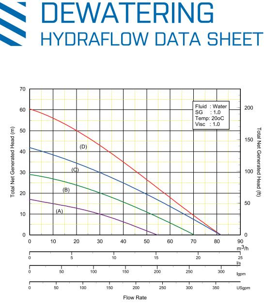
Hydraulic Input: (A) 22 I/m @ 69 bar (B) 25 I/m @ 114 bar (C) 38 I/m @ 158 bar (D) \* 45 I/m @ 158 bar \* Typical performance with HT25D
