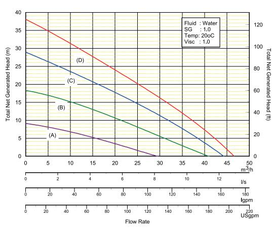
Hydraulic Input: (A) 8 l/m @ 76 bar (B) \* 11 l/m @ 120 bar (C) 15 l/m @ 151 bar (D) \*\* 19 l/m @ 172 bar Intermittent \* Typical performance with HT6D \*\* Typical performance with HT11D
