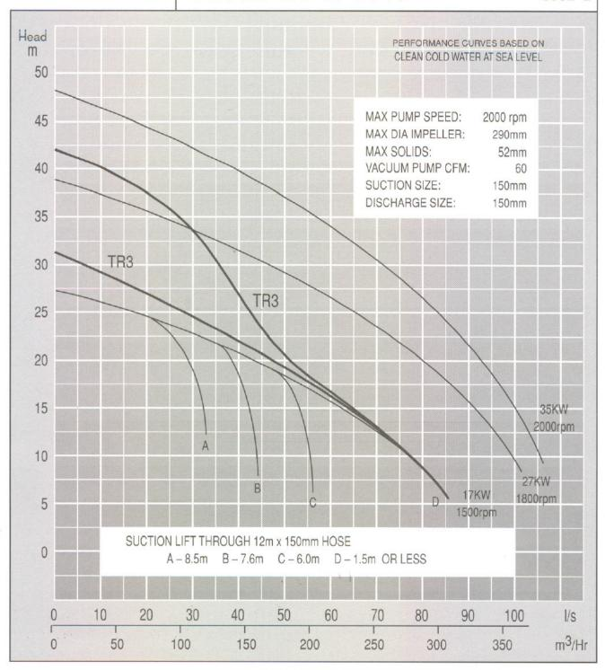
Volute Angle discharge, Horizontal suction. Cast Iron. Impeller 2 vane Open. Cast Iron. Wear Plate SNG Cast Iron. Pump Shaft Steel (BS970 EN8B). Bearings DE: Twin Taper Roller NDE: Cylindrical Roller. L<sub>10</sub> Life: 40,000 hrs at 2000rpm (BEP).
