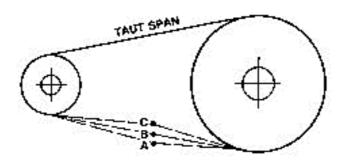
A-C = Total Possible Mid-Span Movement A-B = Depth of Horizontal Free Sag
