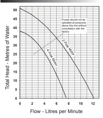
Note: Performance shown is for a new pump fitted with a Neoprene impeller pumping water at 20°C, performance may vary by up to 15%. Consult factory for performance of alternative impeller compounds.
