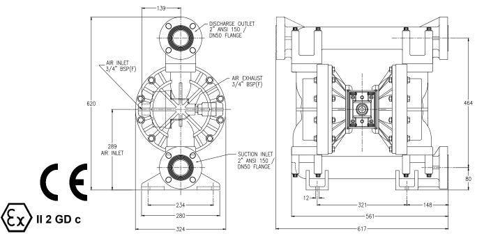
General Assembly :- B50 Moulded Pump, All dimensions +/- 3mm
